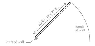
iCADMac provides a variety of methods for defining the size and location of entities. To draw the 12-foot-long wall, for instance, you can specify its starting point, its length, and its angle to other walls. like this:
