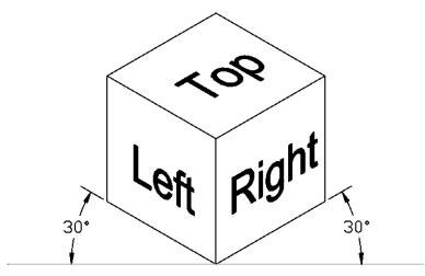
Lines and text are drawn in three isometric planes. (Isometric planes are often named "isoplanes.") The curious thing is that text and dimensions must be slanted by 30 degrees to look correct. You learn how to create isometric text and dimension styles in this chapter.
