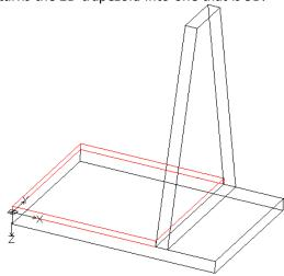
4. Add the square box, which has a 1x1" base and is 1.75" tall. It is located at the center of the end of the main plate. Place it with the coordinates listed below, and then use the **Length** option to specify its size:
