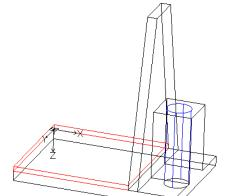
4. To show that the hole now exists in the model, use the **RollView** command to twist the model around.
