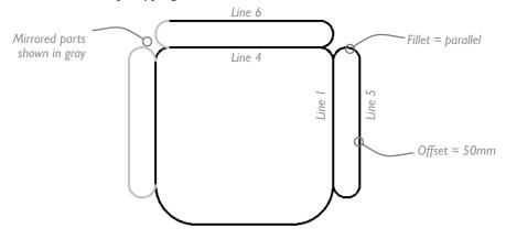
a. To begin drawing the arms and back, start the **Offset** command to create offset parts of the chair seat:
