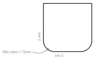
5. The seat has two more fillets, but of a different radius. First, though, use the Multiple option to make the command repeat itself:
