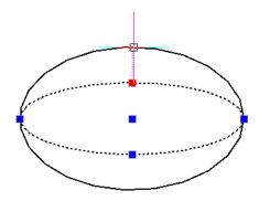
Left: The center grip moves the ellipse. Right: The edge grip stretches the ellipse.
