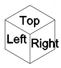
The solution is to slant text by 30 degrees in two directions, obliqued and rotated. *Obliqued* means each letter is slanted, *rotated* means the entire word is slanted, as well. Below, I have applied both angles to the text, making it look correct.
