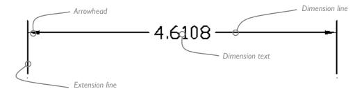
**Extension lines** point to the start and endpoints of the distance being measured.
