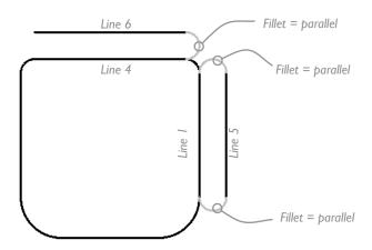
4. Because the chair symbol is symmetrical, you don't have to draw all of the back and arms. These parts can be completed by mirroring existing lines and fillets with the Mirror command. In addition to knowing the entities to be mirrored, this command needs you to specify two points that define an invisible line — called the "mirror line" — about which the entities are mirrored.
